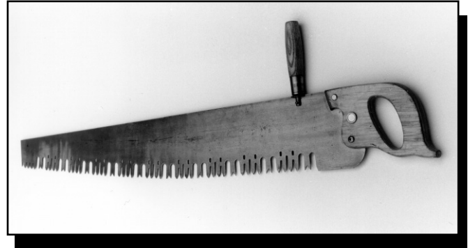
Figure 77—A one-person crosscut saw is a good choice for back-country settings.
