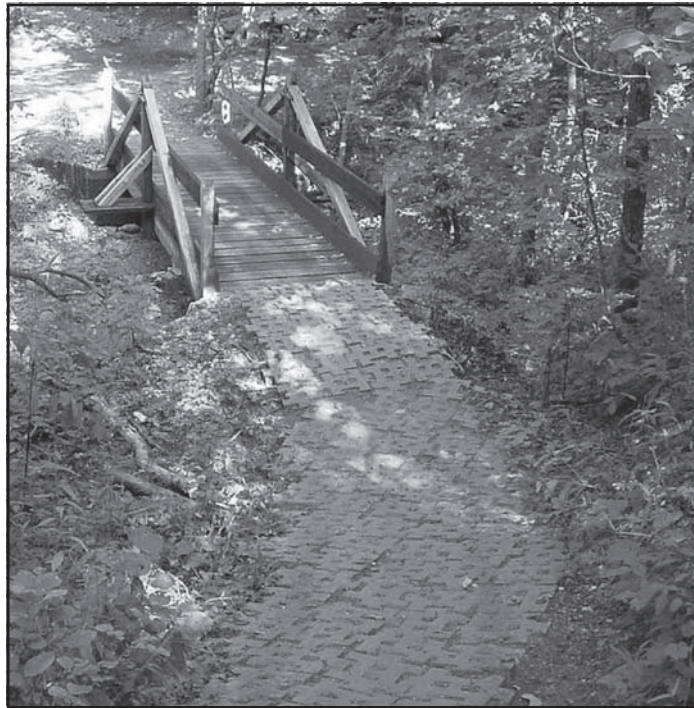
Figure 85—Pavers can be used to armor sections of trail for motorized traffic.
