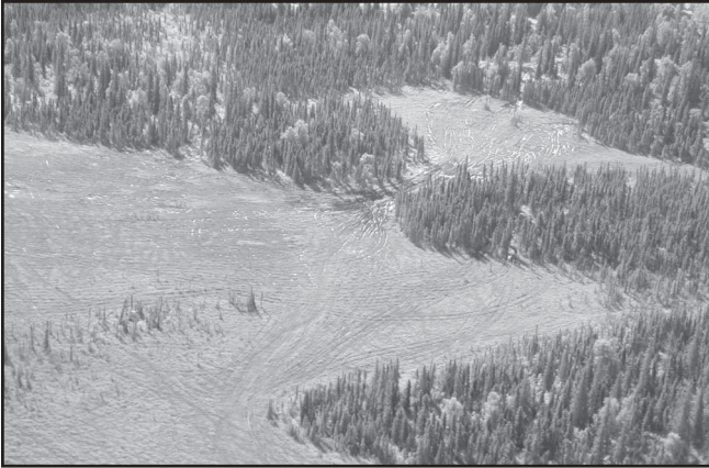
Figure 5—A braided trail in Alaska. More than a dozen separate routes have been pioneered in this section crossing a wetland. Note the wet trail conditions and numerous potholes. At this site, trail impacts affect an area more than 250 feet wide. Braiding significantly extends the area of impact by modifying vegetation cover, surface hydrology, and soil characteristics.
