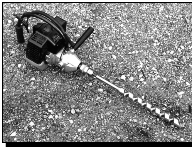
Figure 85—Gasoline-powered drills are great for backcountry work if regulations allow their use.
