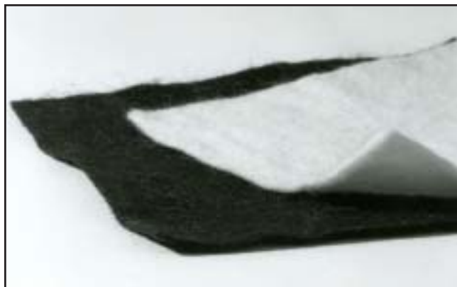
Figure 1—Geotextiles. Felt-like products are easier to work with than heat bonded, slit film, or woven products that have a slick surface texture. They are easier to cut and their flexibility makes them easier to place on curved trail sections.
