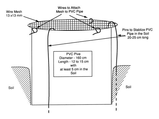
Figure 3-Large acorn protector used at the Pennsylvania State University.
