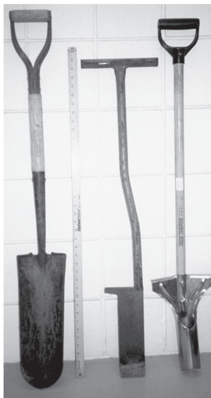
Figure 8.8. Bare-root seedlings can be planted using a sharpshooter shovel, dibble bar, or bulb planter.
