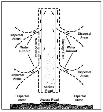
Figure 3. Example of a water turnout that disperses runoff onto vegetable areas. (FI. Dept. Agric. Cons. Serv. 1993)
