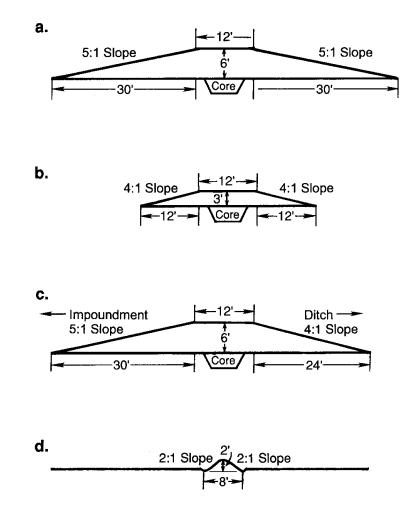
**Fig. 1.** Dimensions of levee for a permanent or semipermanent impoundment (a), levee for a seasonally flooded impoundment (b), header-ditch levee (c), and rice-dike levee (d).
