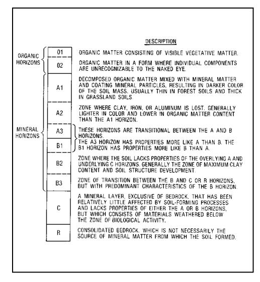
Figure 2. Generalized soil profile
