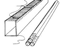
**Fig. 2.** Three designs for beaver-proof water control structures: three-log drain (*top*), box drain (*lower left*), and perforated plastic drainpipe (*lower right*). From Arner and Hepp 1989.
