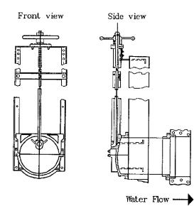
**Fig. 2.** Stoplog (a) and screw gate (b) water-control structures for manipulating water levels.
