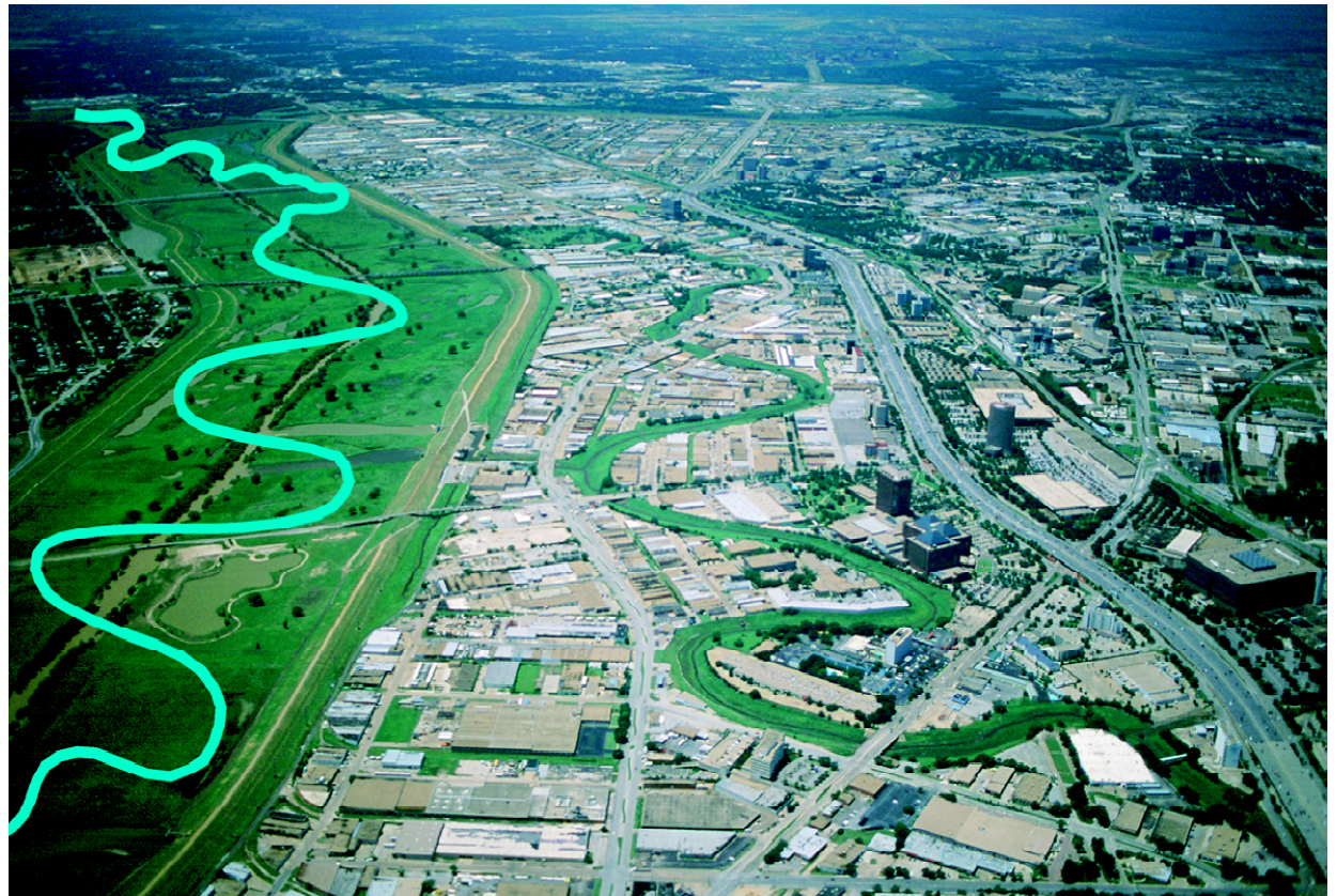
Conceptual diagram illustrating how the sinuosity of the Trinity River may be partially restored. A remnant of the original river alignment, "The Meanders", is clearly visible in the right side of the photo.
